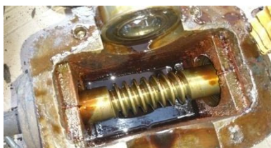
Figure 2. Gear box having worm gear
